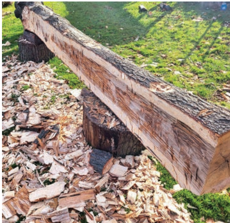
After most of the material is removed, a bit of fine tuning and trimming back to the line is all that's left. The other side gets the same treatment, then rotate the log onto a flat side and repeat. You can see how flat and straight a log can be made, along with the tell-tale marks of a hand-hewn beam.
